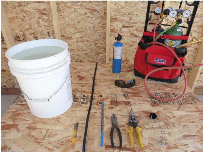
Demonstration: Take a used hacksaw or reciprocating saw blade and show or allow the students to see or feel its properties when handled, flexed and moved. Steel banding will work also but the effects are not as dramatic. The metal will always spring back to its original shape.
