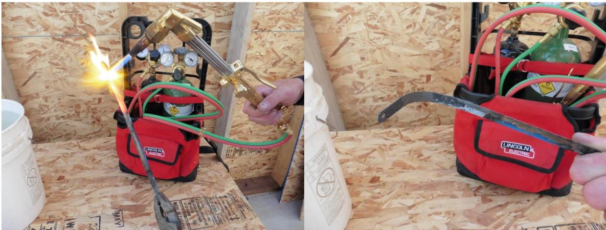
Next temper the hacksaw blade: You can use the same blade. Heat the blade up again to a bright orange color and quickly quench it in water. Now you can take it and break it with your bare hands or hit it with a hammer and it will shatter. Now it has been tempered.
